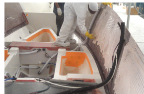
Large FRP laminates: Prepping hull to bond liner
