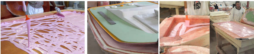
Applying Standard J-Core to the hardtop shell
