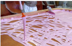
Applying J-Core to the hardtop shell
