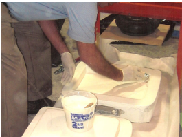
WET OUT FEMALE HALF Using 1.5% clear or disappearing red MEKP
