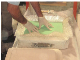
ADD CORE & GLASS press core, add more glass and remainder of 4901
