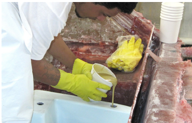
Using foam in aft hull to prevent 6011 from escaping during transom pour
