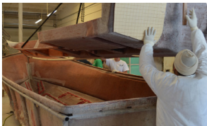
Bonding stringer assembly to prepped hull
